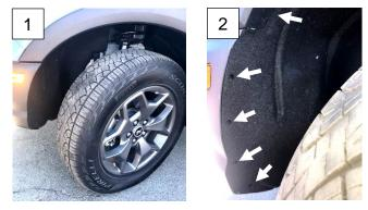
2. With the trim tool, or flathead screwdriver, remove the five plastic fasteners in the front of the driver side wheel well. With the 7mm socket, remove the single fastener on the underside of the bumper.
