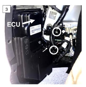
4. The last fastener holding the ECU onto the mount will need to be removed by reaching through the driver side tow hook opening and removing the nut with the 10mm wrench. A detailed view into the tow hook opening is shown below. The upper circled location is the mount and the lower circled location is the stud.
