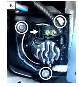
6. With the three OEM fog light screws from step 5, mount the driver side Baja Designs S1 fog light bracket. Leave the S1 light off until the next step.
