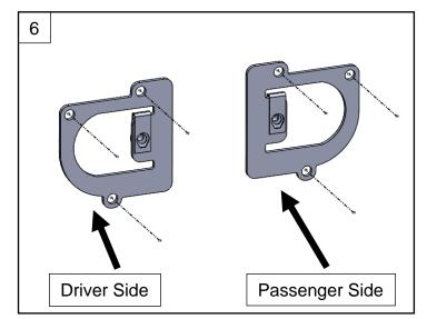
7. With the 3mm Allen wrench and two of the small pan head bolts, mount the S1 bracket to the driver side light.
